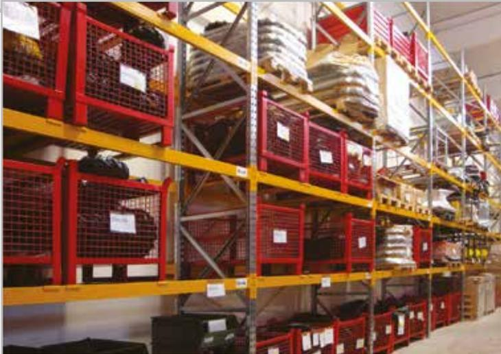
Shelving System that can be modulated with Earthquake proof Structure, planned and certified for every use according to the different storing necessities.
